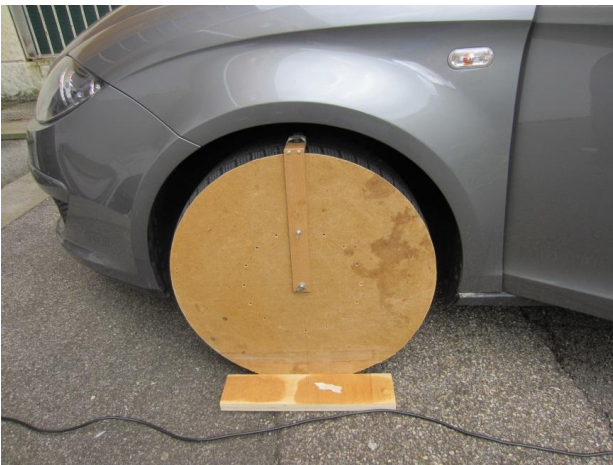
Fig. 1. Transmitter located on the wheel [0, 0, 30] cm. Origin of the coordinate system is the center of the front-left wheel
