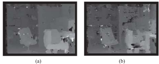
Fig. 20. DE results using the rectified images of CLUT-R (a) DE result of mini-census [2] (b) DE result of AWDE [4].
