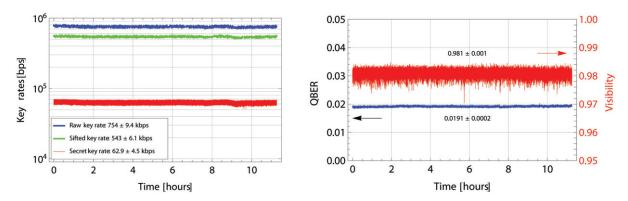
**Figure 6.** Key rates (left), QBER and visibility (right) demonstrating the stability of an autonomous QKD run for a period of more than 11 hours. Alice's and Bob's devices were connected by a single 12.5 km fibre. The secret key rate (left, red) accounts for finite-key effects, the authenticated key rate (left, purple) for the consumption of secret keys to encrypt the authentication tags.
