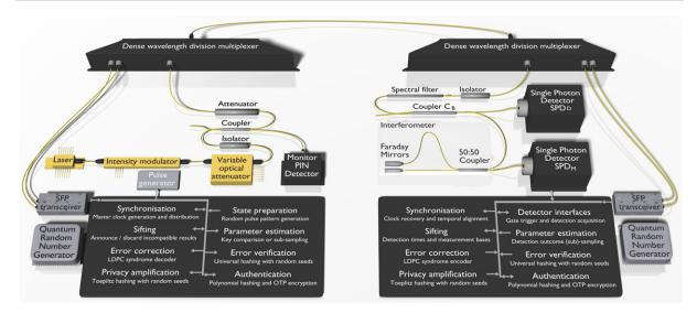
**Figure 1.** Schematic representation of our optical implementation for the COW QKD protocol and the key distillation procedures implemented in the fast FPGA hardware.
