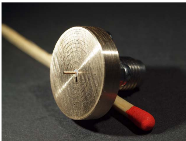
Figure 3 Ground plane with connector pin extension, Teflon washer and 1.85 mm connector on the back. [Color figure can be viewed in the online issue, which is available at wileyonlinelibrary.com ]
