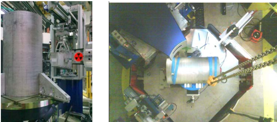
FIG. 1: billet section positioning for measuring the radial and hoop (left at Salsa) and axial (right at Poldi) strains. The weight of the billet sample is 130kg.
