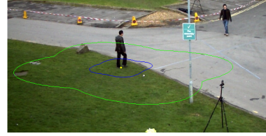
Figure 3: The iso-contour of value 0 of the \beta surface for the position model for \Delta = 3 (blue) and \Delta = 15 (green), centered around one detection.
