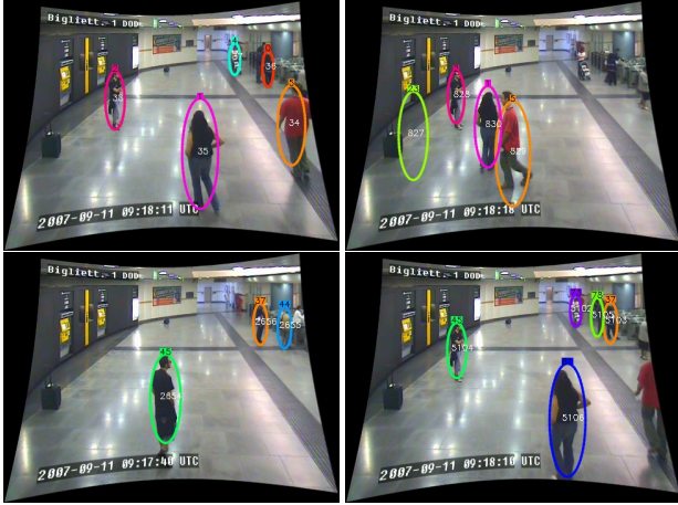
Figure 8. Examples of tracking output on typical surveillance data from a Torino metro station (each row is taken from a different sequence)
