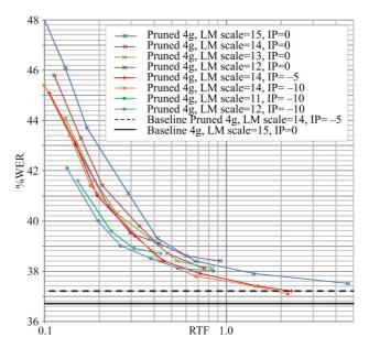
Fig. 5. Real-time factor (RTF) against %WER on *rt07seval* IHM for various decoding arrangements with HTK HDecode and Juicer. "Baseline" refers to lattice generation with a bigram LM and rescoring with a 4-gram LM.
