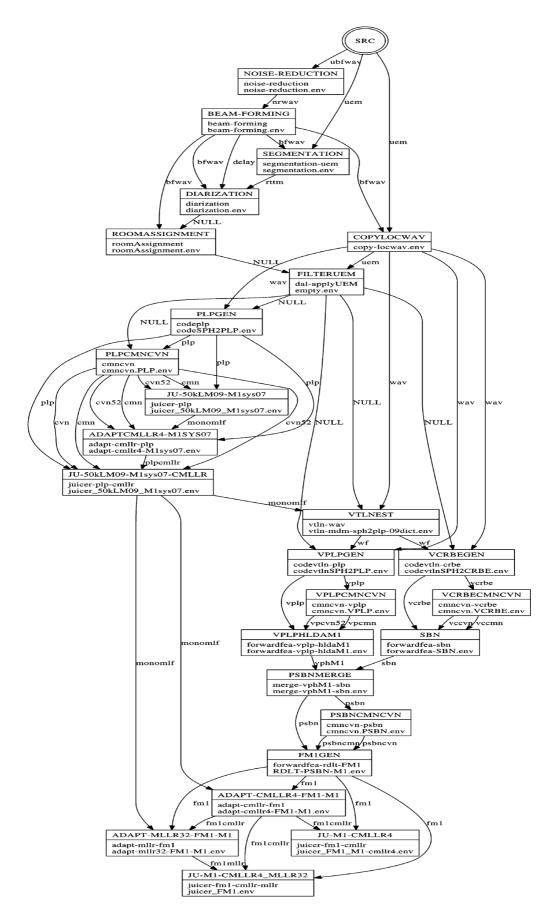
Fig. 8. Graph of the 2009 MDM system. Arcs describe data types; NULL indicates transport of metadata only. Boxes hold module instance, module, and configuration names.
