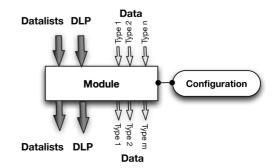
Fig. 7. ROTK modules. Data lists hold metadata such as speaker or segment information, DLP files list data lists and processing information.
