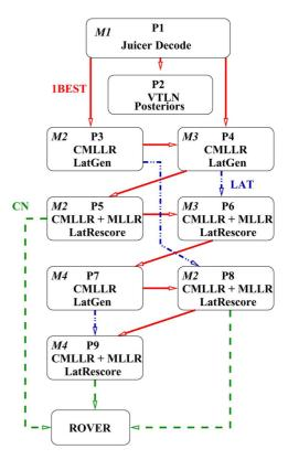
Fig. 6. AMIDA RT'07 system schematic. LatGen denotes lattice generation, LatRescore acoustic rescoring.
