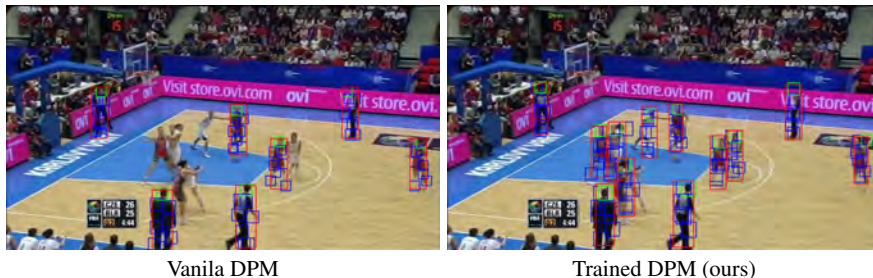
Fig. 7 Detection results of the DPM trained using only the INRIA pedestrian database (left) vs. our retrained DPM (right). In both cases, we use the same parameters at run-time and obtain clearly better results with the retrained DPM.
