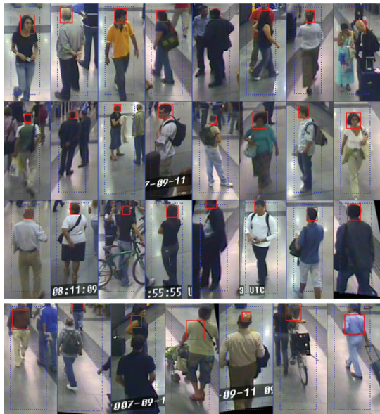
Figure 4. Head localization results. Dashed blue box is the human detection output. Solid red box is the head localization outputs (first candidate). Failures are shown in the last row
