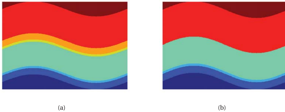
Figure 6.1: (a) Schematic view of a cell with buffer layer; The layers are ITO, p-Si, i-Si, n-Si, ZnO and Ag respectively, (b) The same cell when there is no ZnO buffer and n-Si layers. Light comes from below and the back-reflector is on top
