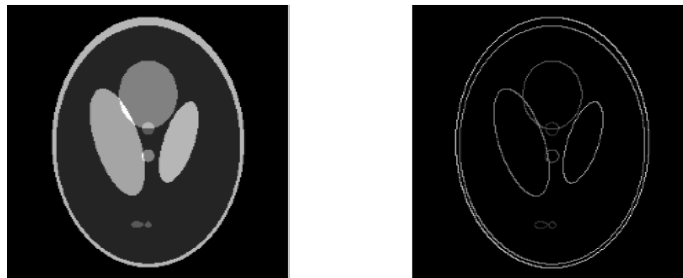
Figure 1: (Left) 256 \times 256 Sparse Gradient Shepp-Logan phantom image. (Right) Nonzero horizontal and vertical discrete gradient information.
