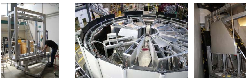
Figure 13: The prototype before (left) and after (middle) installation in the MARS tank. In the right panel all of the shielding elements are mounted (side walls, walls between the banks, slits between analysers and detectors, and a slit between the sample and the first analyser).
