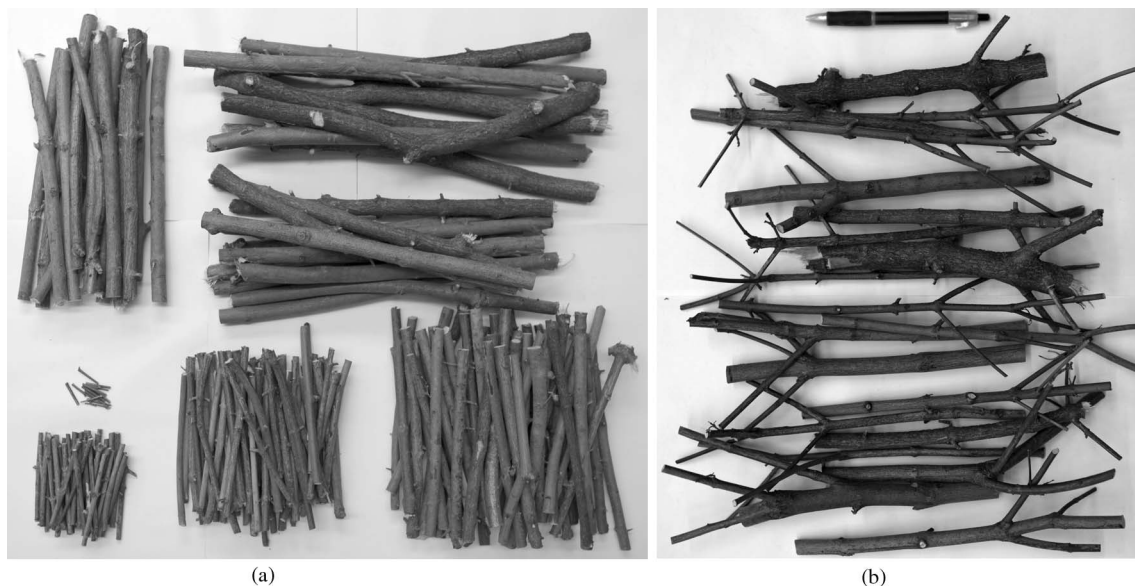
Fig. 4. Model debris including (a) trunks (size classes according to Table 2); and (b) rootstocks (Table 3)
