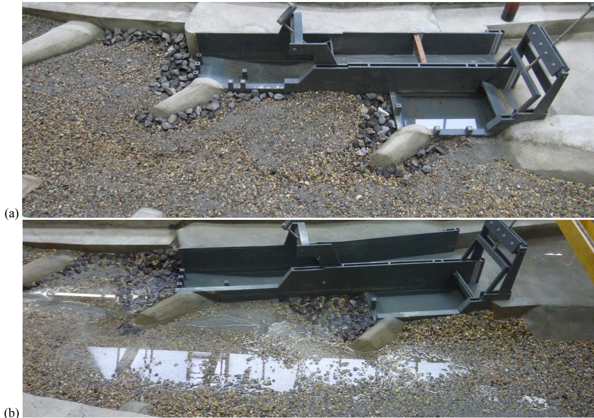
Figure 5 Physical model of G1, (a) with lateral baffles, and (b) without
