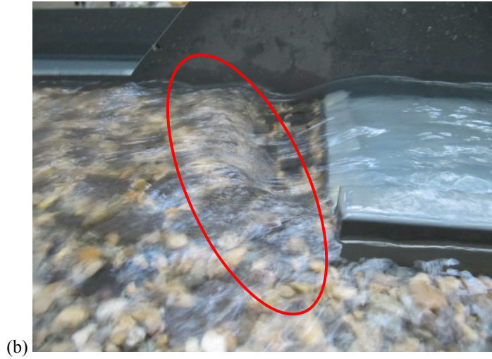
Figure 8: Hydraulic jump downstream of the the stilling basin end sill due to insufficient energy dissipation in the stilling basin. Observed hydraulic jump for an outlet discharge of Q_B=60 \text{ m}^3/\text{s} and a river discharge of Q_A=5 \text{ m}^3/\text{s} , for (a) a riprap located at the same level as the end sill, and (b) a 0.5 m lowered riprap elevation
