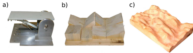
Fig. 4. Pictures of the three different terrain sample types for the experiments (a) adjustable incline for preliminary testing, (b) terrain sample with simple geometry and (c) naturally inspired sample with a complex shape.
