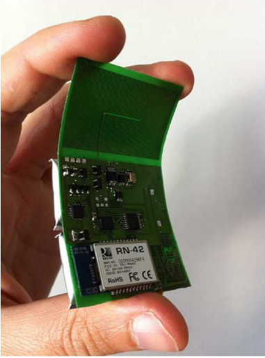
Fig. 1. A system is designed to power implantable sensors through an inductive link. The system is realized on a flexible substrate to be embedded into a skin patch and is used to test multi-layer receiving inductors. Reprinted from [16].
