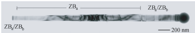
Figure 11. A TEM image of a GaAs NW grown for 40 min with a V/III ratio of 8 and a pyrometer temperature of 635 °C at GR_{\text{planar}} = 0.3 \mu\text{m h}^{-1} . The distribution of TPs appearing at the bottom and at the tip is typical of Ga-catalysed GaAs NWs. The structural distribution depends on the relative size of the liquid phase (which changes during growth, see figure 12) because the latter has a huge influence on the nucleation statistics (see sections 2 and 4).
