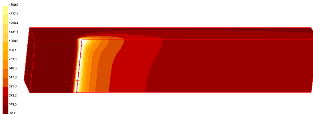
Fig. 10. Steady state temperature distribution (temperatures lower than 1500 °C).
