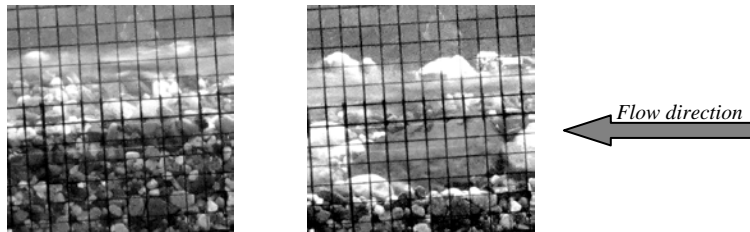
Figure 3 Example of fast erosion around a boulder, at instant 693 min and 694 min.
