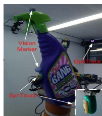
Figure 17: Implementation of a computed grasp for the flask bottle on the Barrett hand.
