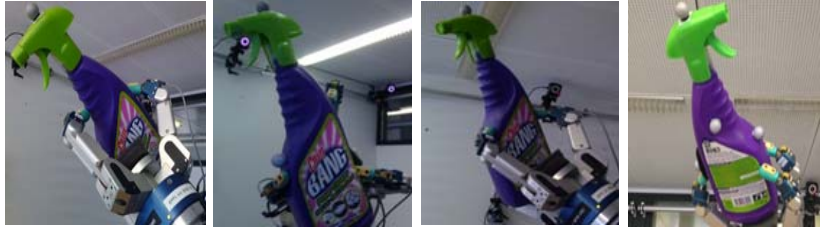
Figure 18: Implementation of several grasps generated for the flask bottle on the Barrett hand.
