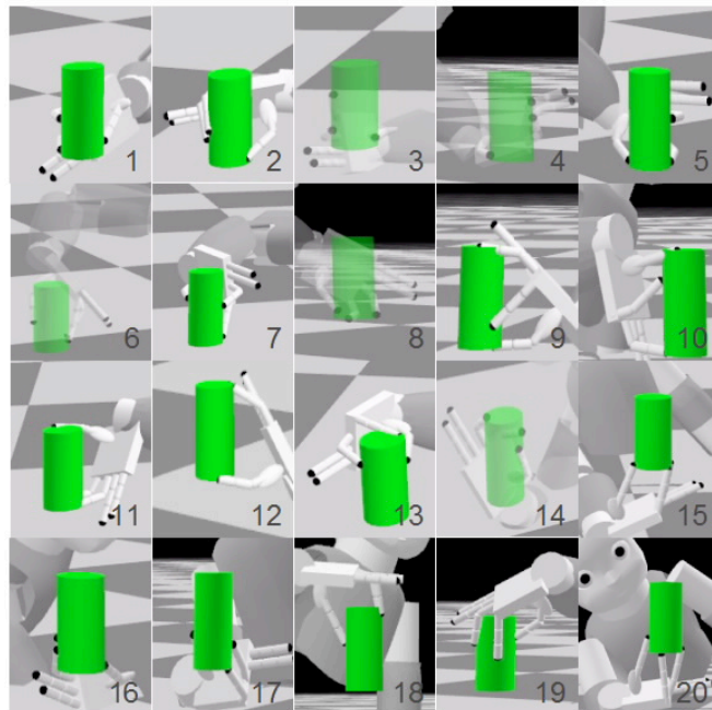
Figure 11: The different iCub hand configurations to grasp a cylinder, labeled from 1 to 20.
