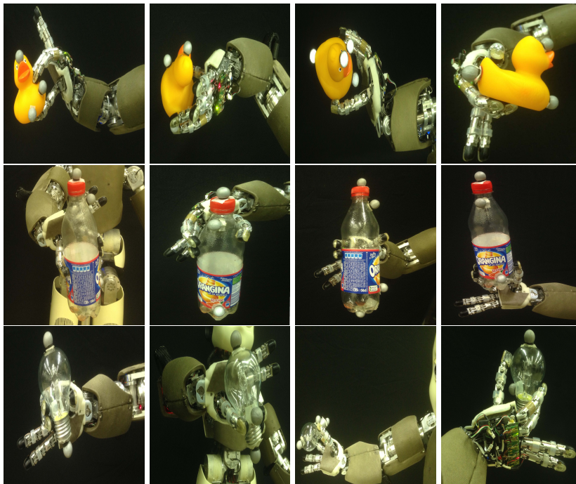
Figure 19: Grasps computed for the iCub hand on some real objects modeled with Gaussian Processes.
