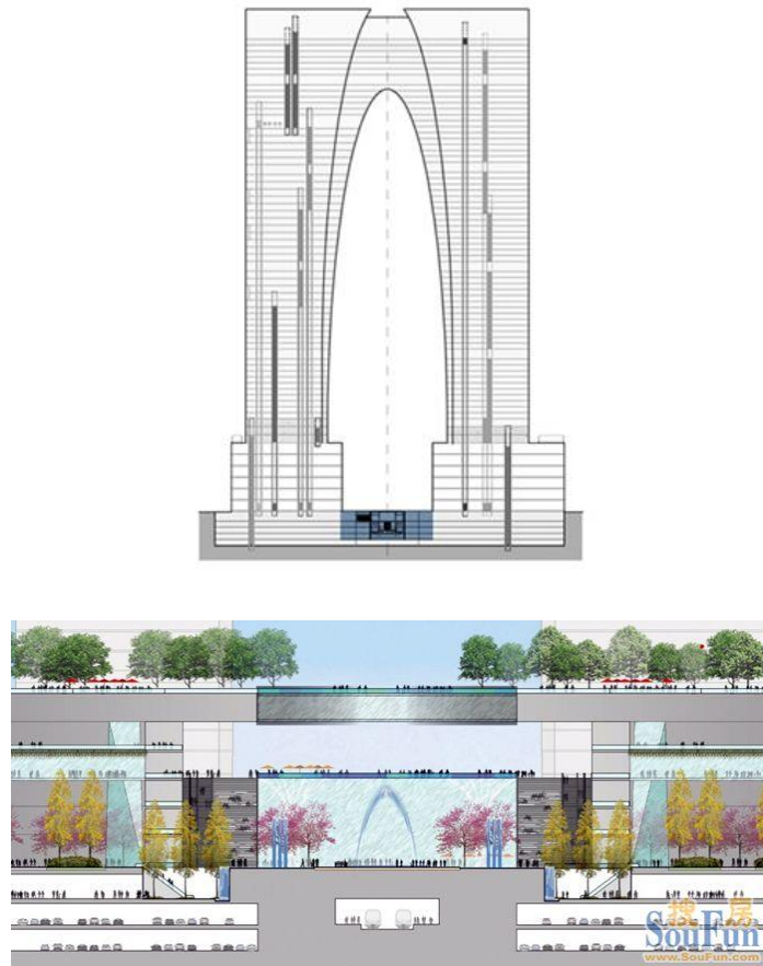
Figure 3:24 The Orient Gate underground complex: commercial basement + subterranean station + metro tunnel (total floor space: 500,000 square meters)
