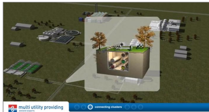
Figure 1:3 Example of Dutch multi-utility tunnel: Multi Utility Providing (MUP), Smart Link, The Netherlands 1
