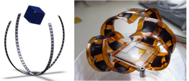
Fig. 4. Concept diagram and proof-of-concept of DEMES gripper.
