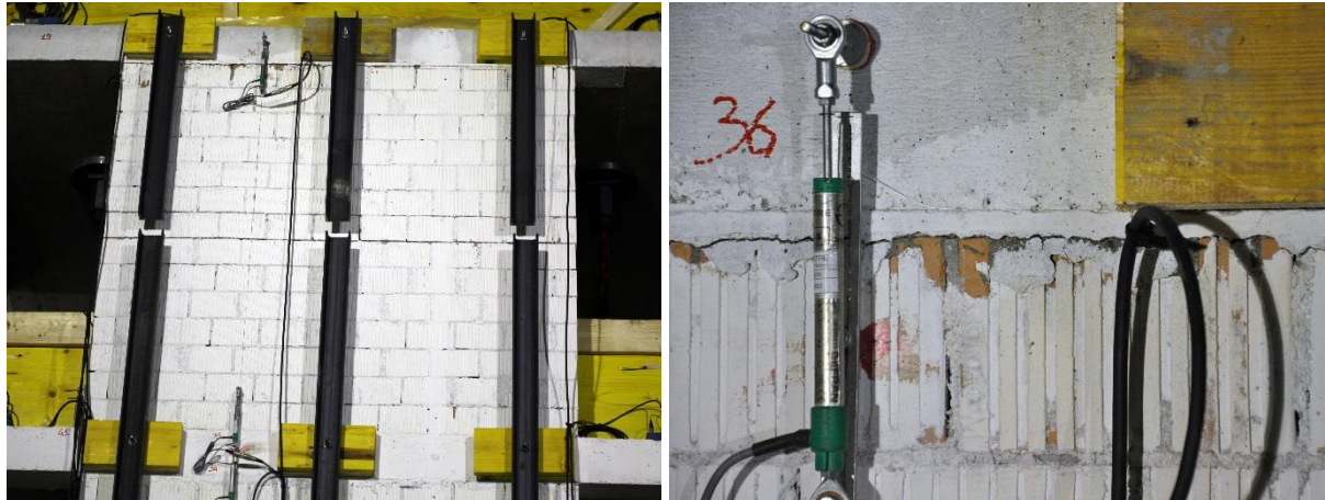
Figure 10. Out-of-plane failure of URM wall: horizontal cracks at mid height and on top of the wall.
