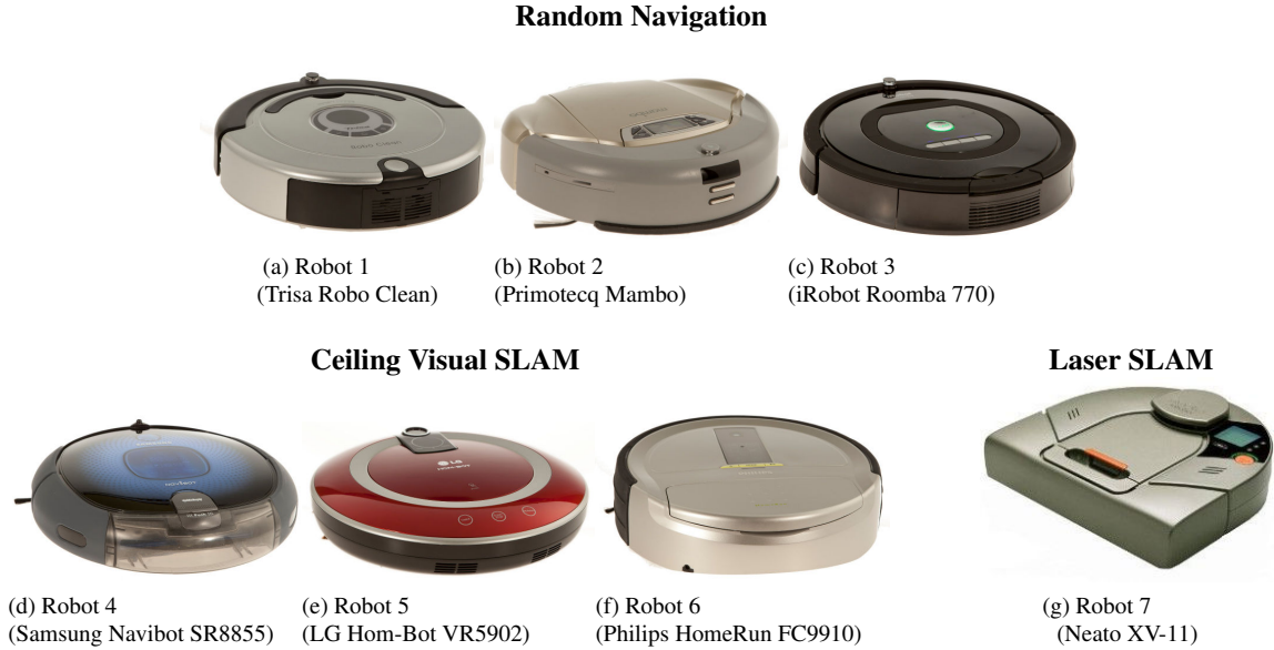
Figure 2: Robots used for the technical study, sorted by their localization technology. Copyright for (a) to (f): RTS / ABE; for (g): Neato Robotics.
