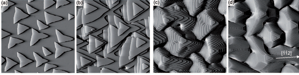
Figure 2.7: STM images of the early growth stages of Pt(111), taken from Krug [76].
