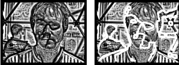
Figure 4.22 : Normalized feature image following Method 5 (left), same with corresponding shadow mask (right).
