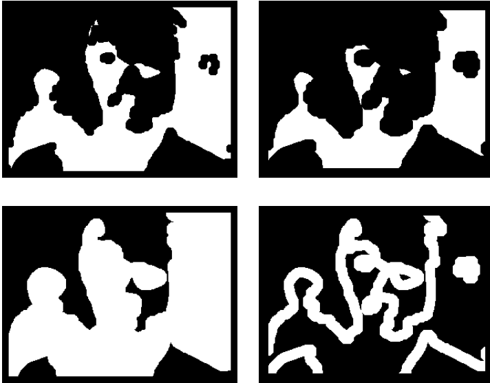
Figure 4.19 : Shadow mask construction for Method 4. Initial mask (top left), eroded mask (top right), dilated mask (bottom left) and shadow mask (bottom right). The shadow mask corresponds to the difference between the dilated and eroded masks.
