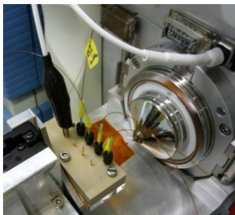
Figure SI-2. SPE-GEMS microchip is placed in front of the ESI-MS source inlet.
