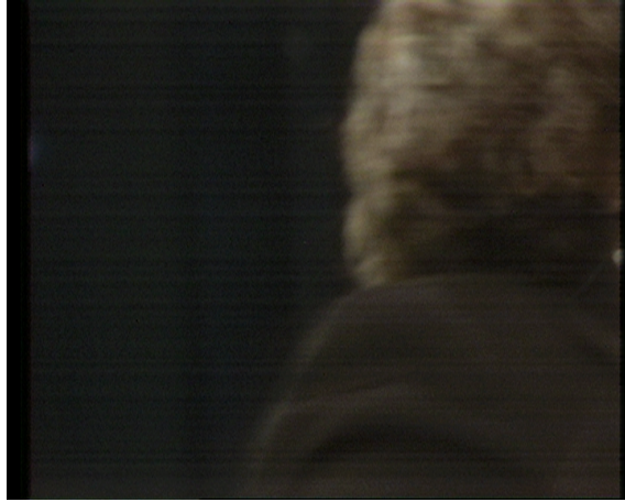
Figure 3: Horizontal lines due to dirty heads on videotape recorder.
