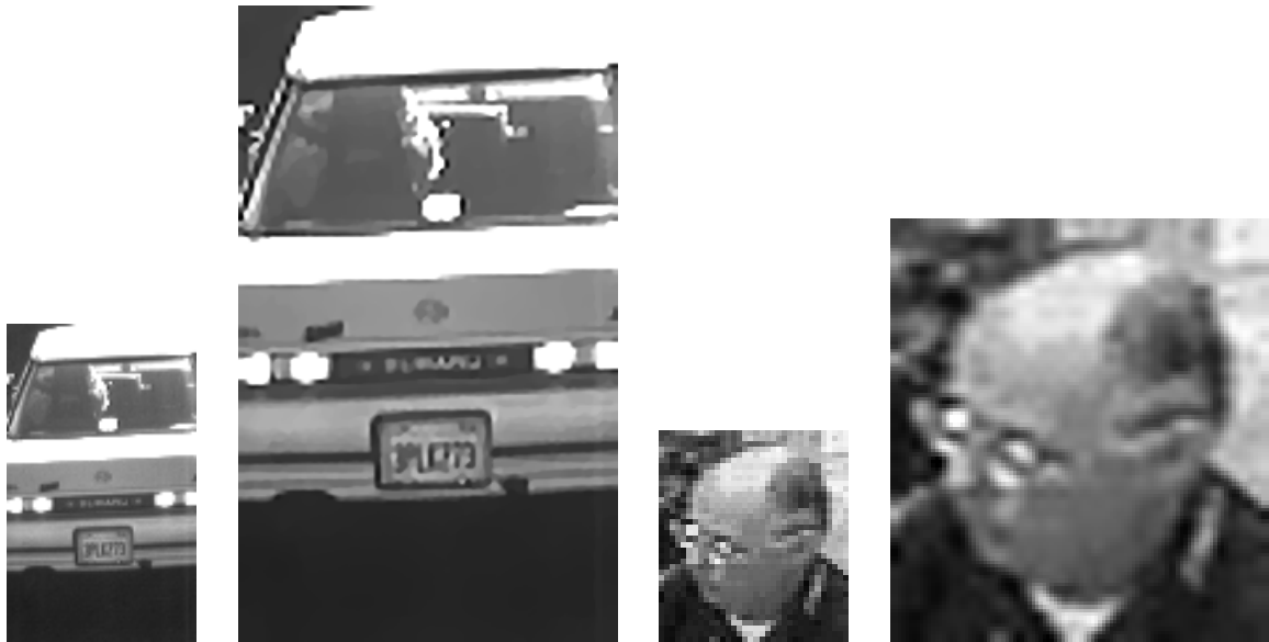
Figure 3.12: Results in the noise free case. In both experiments, we used a zoom factor of 3 along each dimension and patches of size 5-by-5 pixels.
