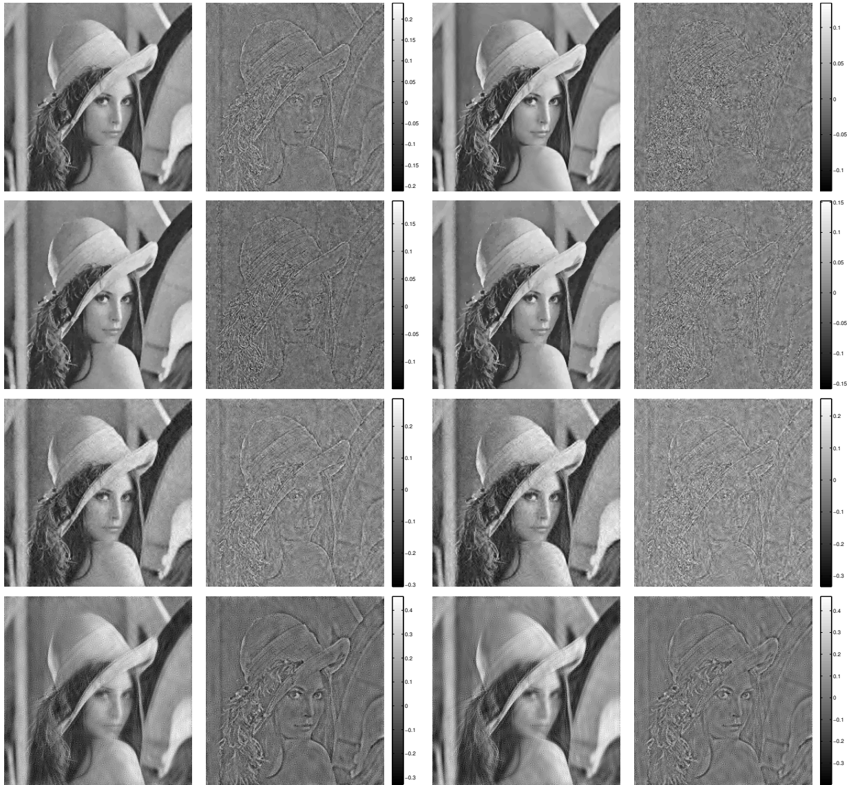
Figure 2. Reconstruction example of Lena for spread spectrum acquisition, with M = 0.2N and input SNR set to 30 dB. First and third columns show the reconstructed images and the second and fourth columns show the error images. First row: BPSA(24.4 dB) and SARA (27.9 dB). Second row: TV(26.3 dB) and RW-TV (26.6 dB). Third row: BPD8 (21.4 dB) and RW-BPD8 (21.2 dB). Fourth row: Curvelet (18.7 dB) and RW-Curvelet (18.3 dB).
