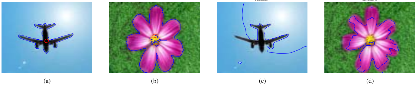
Fig. 6. Segmentation of color images with HAC model and a the convex formulation of GAC+ACWE models. Initial level set set in red, final segmentation in blue. Note that initialization does not affect the convex GAC+ACWE segmentation model. (a) HAC 11.6s. (b) HAC 25s. (c) GAC+ACWE 1.5s. (d) GAC+ACWE 2.1s.
