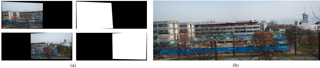
Fig. 5. (a) Prealigned captured images and their masks; (b) photo-mosaic of EPFL campus created using the proposed MBB implementation
