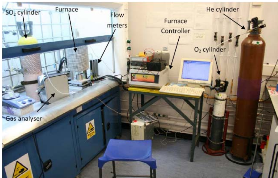
Figure 13 Experimental setup for high temperature membrane testing (see online version for colours)
