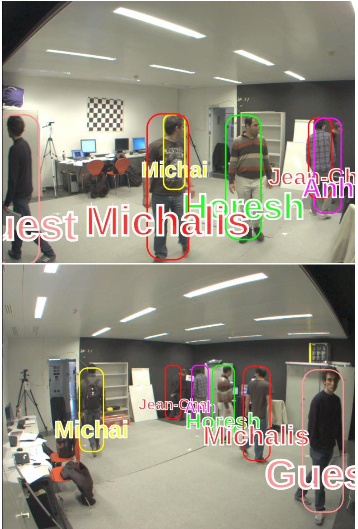
Figure 33 - Screenshot of the tracking results from 6 people video sequence as seen from cameras 2 (top) and 3 (bottom). Everybody in the scene is correctly identified. The person marked as a “guest” isn’t saved in the database, consequently he isn’t recognized throughout the video.
