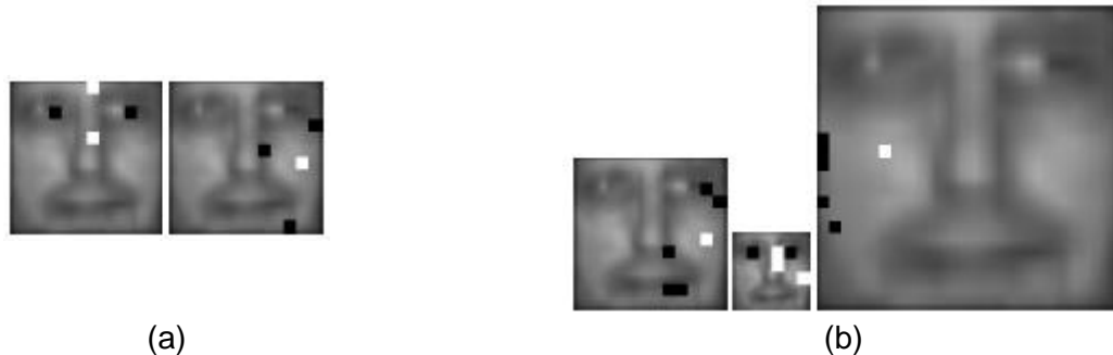
Figure 3 - The features of the first two layers of the cascade classifier overlaid on image patches (from [3])
