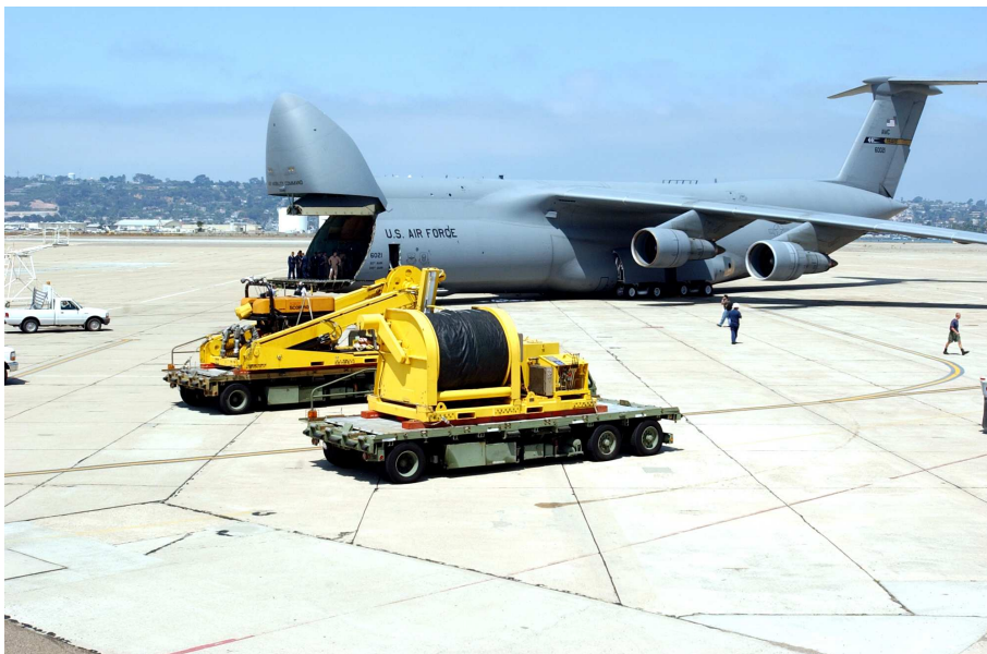
Figure 2.2: A SuperScorpio ROV is being loaded into a Galaxy for a submarine rescue mission in Russia. The trailer in the foreground carries the umbilical cable.
