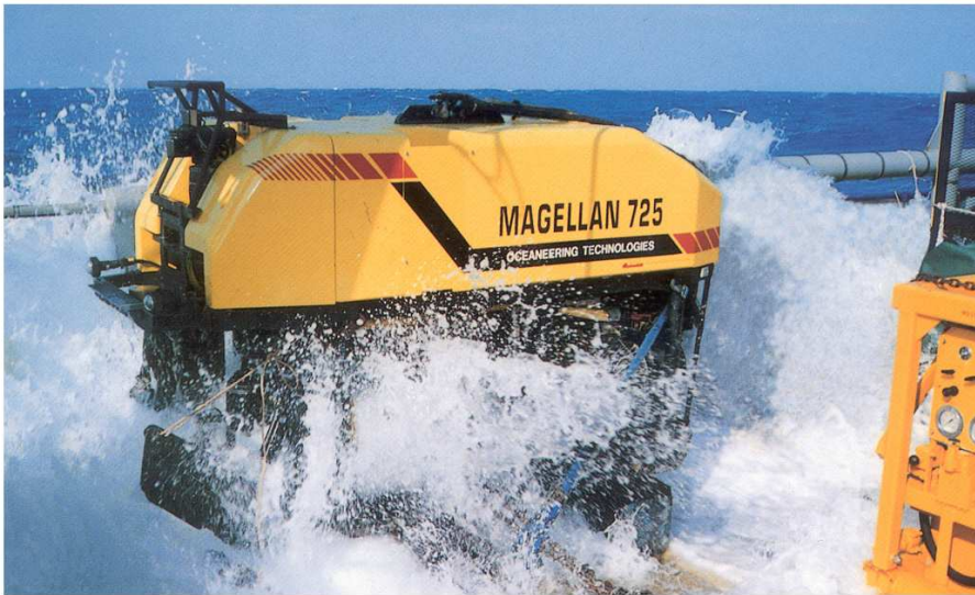
Figure 2.1: A Magellan ROV being launched into the Ocean
