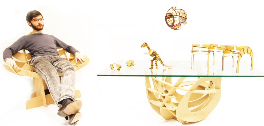
Figure 1: 3D designs composed of planar intersecting pieces fabricated using laser cutting and CNC milling.
