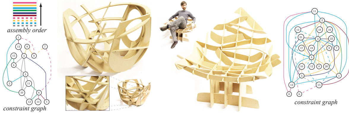
Figure 10: The base of a coffee table and a freeform chair milled from medium density fiberboard (MDF) (see also Figure 1). Complex joints like the one illustrated in the zoomed image can easily be created with our method. The design graphs illustrate the complex coupling of constraints. The parallel cut sets computed by the optimization are indicated by color in the order of assembly. The smallest intersection angle is 50^\circ , as mandated by the CNC milling machine.
