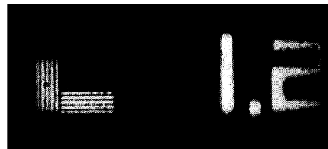
Fig. 6 Test pattern imaged with a single melting resist microlens ( \Phi=250 \mu\text{m} , \text{NA}=0.36 ). A resolution of 400 lines/mm ( 1.2 - \mu\text{m} feature size) is observed in a microscope under white-light illumination.
