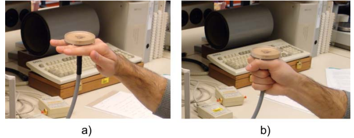
Figure 7: TKA antenna measured while held in the hand. Over the open hand surface (a) and over the closed fist (b)
