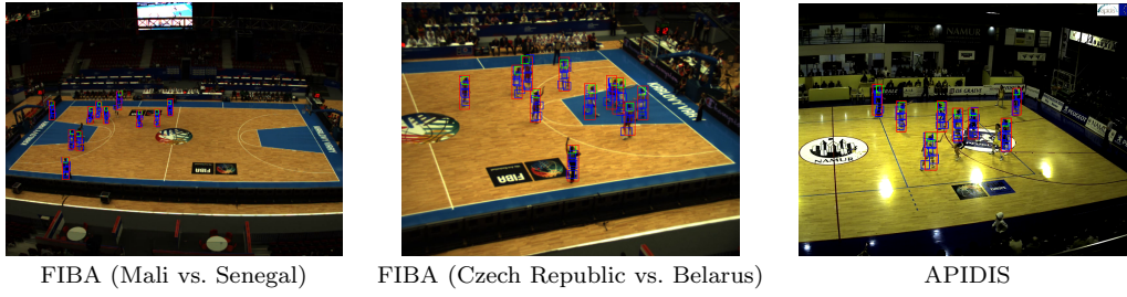
Fig. 4 Representative detection results of our retrained DPM on images acquired using static cameras. We remove detections that correspond to locations outside of the court. The players' bounding boxes are overlaid in red, the head in green, and the remaining body parts in blue. The heads tend to be located much more accurately than the other body parts.
