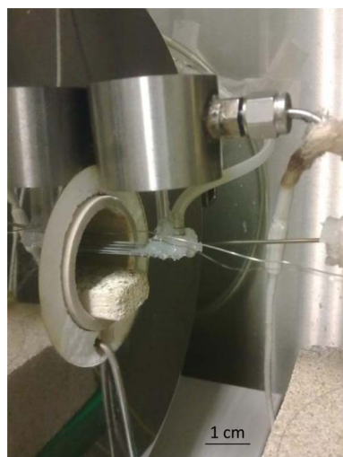
Fig. 2 Measurement set-up for microreformer characterization in external furnace. Gas inlet is outside the furnace in the cold part of the carrier.
