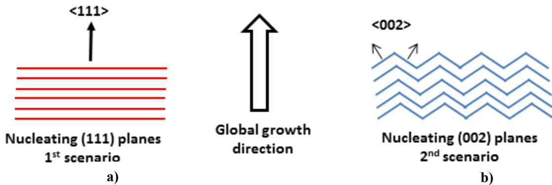
Fig. 2.3: Schematic illustrations of the possible growth configurations of the late stage growth by Je et al.: a) nucleating the (111) microscopic planes, and b) nucleating the (002) microscopic planes [18].
