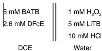
Scheme 3. Schematic representation of the initial composition of the aqueous phase and the organic phase for studying hydrogen peroxide reduction in a biphasic reaction.
