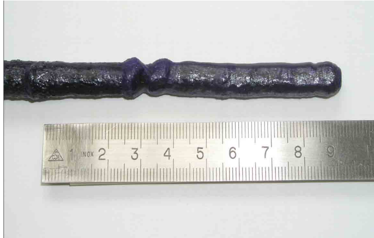
Figure 2.5: Single crystal of \text{SrCu}_2(\text{BO}_3)_2 grown by traveling solvent floating zone technique at PSI. The single crystalline part at the top of growth (right on the figure) is several centimeters long. For neutron scattering studies natural boron was replaced by the ^{11}\text{B} isotope.
