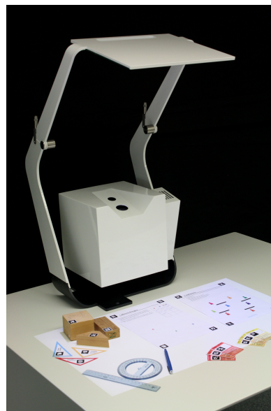
Figure 1: Our camera-projector system on a table, along with various types of objects which can be augmented: sheets, cards, tools and wooden blocks. In Quads, only sheets, cards and cardboard shapes are used.
