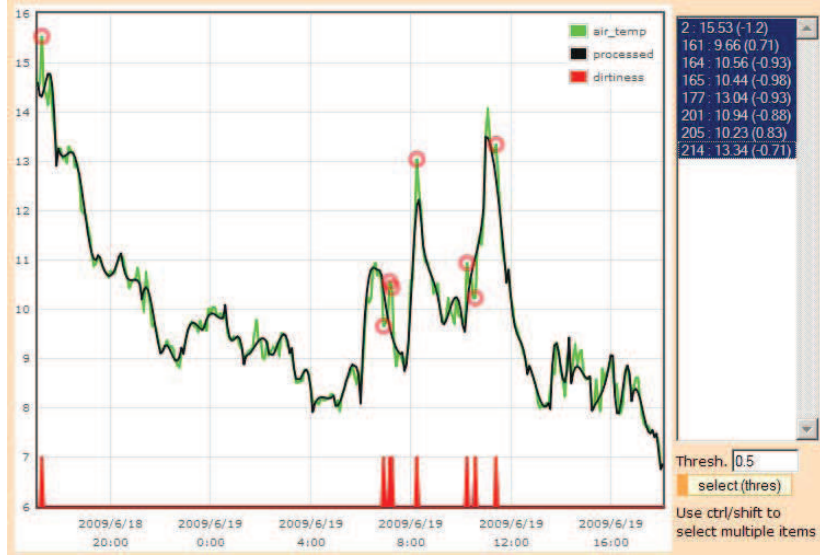
Figure 1.6: Detected anomalies based on 2-degree Chebyshev regression.
