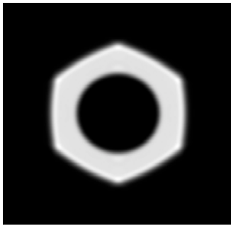
Figure 1 : Calculated far-field of an annular shaped pattern generated by an aperture-modulated diffuser (AMD), KrF-Excimer laser at 248 nm [6].
