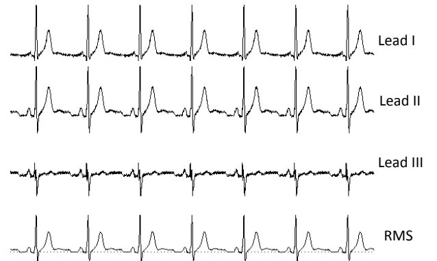
Fig. 4. Three-leads acquisition and corresponding RMS-combined signal.
