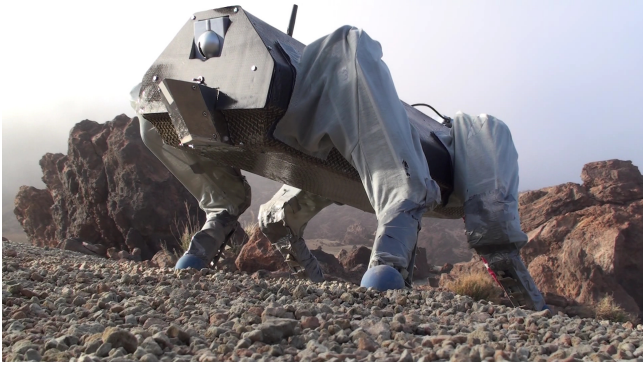
Bild 2: The quadruped robot ALoF. The robot is built with a classically stiff actuation in which joints, gearboxes, and motors are rigidly connected.
