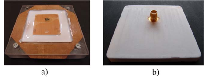
Figure 5. a) Filling the antenna mold with PDMS (visible PDMS penetration through the copper mesh), b) Soft and flexible antenna (bottom side) ready for measurements and use
